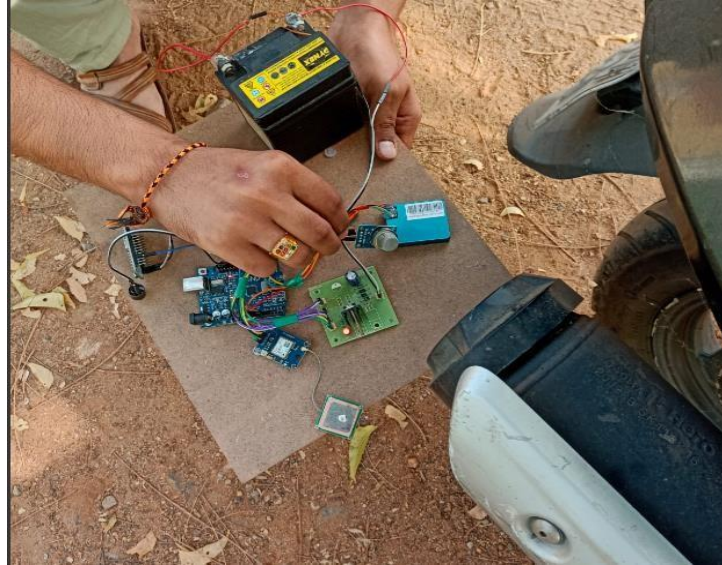
Fig 3. Testing the model by placing it near the exhaust terminal
