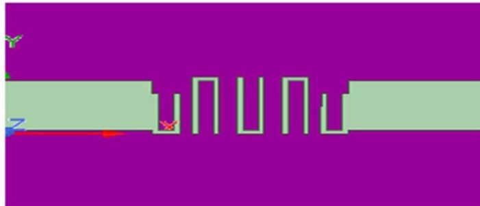
Fig 1: Hairpin Structure arrangement in HFSS
