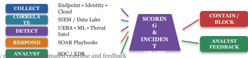
Figure 7: AI-enabled SOC workflow from telemetry collection to automated response and feedback
